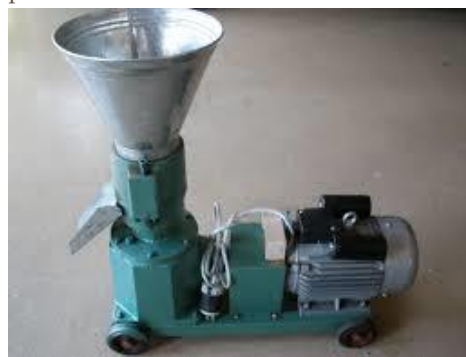
This is an example of a pellet mill which is used to make grass pellets.
